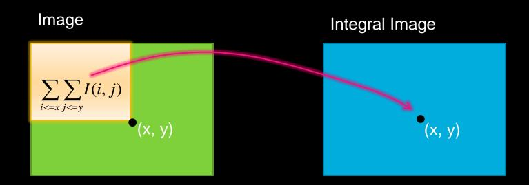
The value of the Integral Image at point (x, y) is the sum of all of the intensities in the gold box. An integral image can be created in a "recursive" manner to minimize computations. Start at the top-left corner and work down a row at a time.
